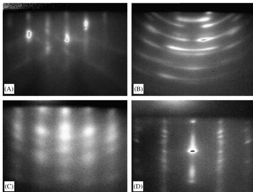
Fig. 2. RHEED patterns for: (A) GaAs substrate after oxide desorption, (B) GaAs substrate after 5 min of nitridation, (C) nitridated GaAs substrate after annealing at 600 °C and (D) GaN film grown at 750 °C.
