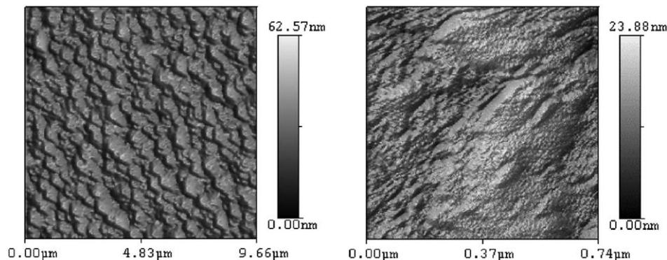
Fig. 4. AFM images of a  $\sim 2\mu\text{m}$  thick GaN film grown on a GaAs substrate.
