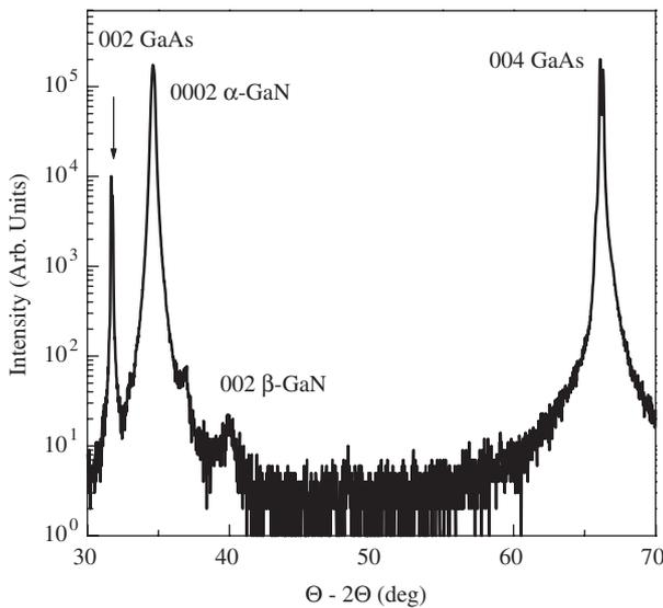
Fig. 3. XRD  $\theta$ – $2\theta$  scan of a  $\sim 2\mu\text{m}$  thick GaN films grown on a GaAs substrate.
