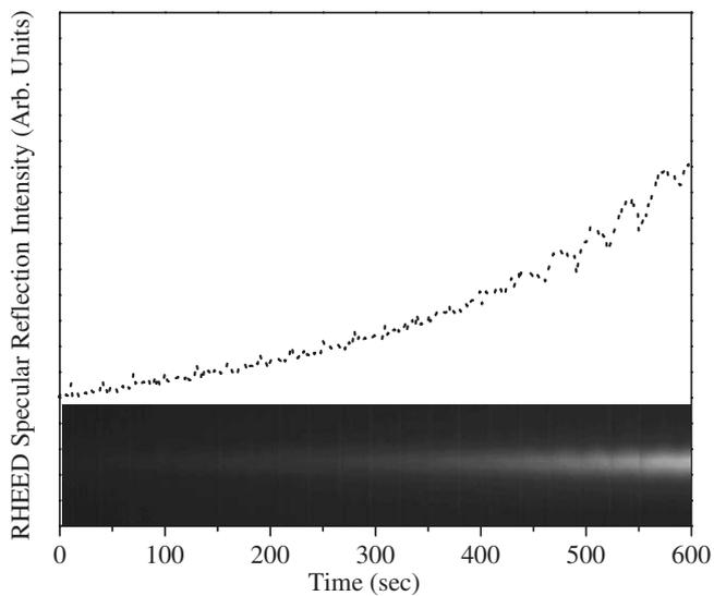
Fig. 1. Time dependence of a specular RHEED reflection.
