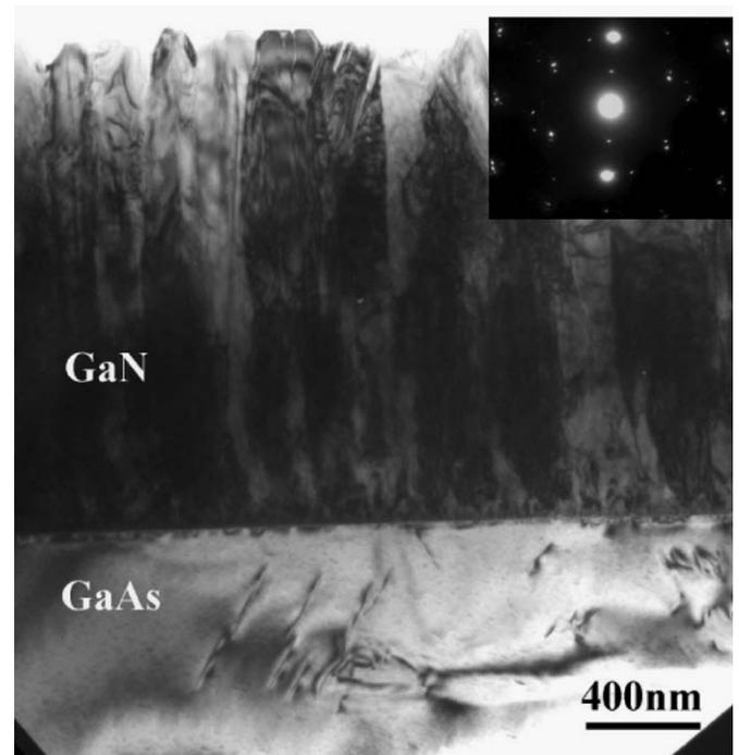
Fig. 5. Cross-sectional bright-field TEM image of a  $\sim 2\mu\text{m}$  thick GaN film grown on a GaAs substrate. The inset is a selective area diffraction pattern.
