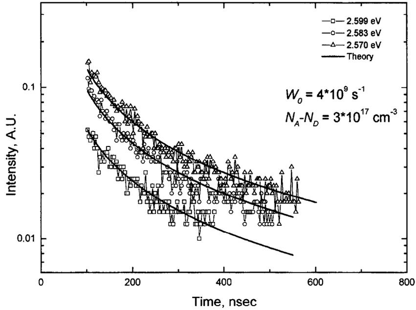
Fig. 2. Time-resolved photoluminescence of Sample C at three different emission energies. Solid curves are the theoretical fit according to Eq. (3).
