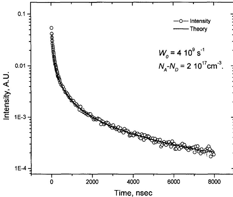
Fig. 1. Time-resolved photoluminescence of Sample D at an emission energy of 2.53 eV. The solid curve is the theoretical fit according to Eq. (3).
