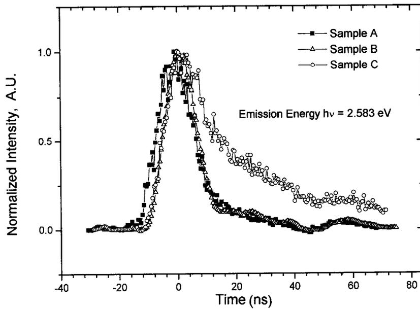
Fig. 3. Comparison of the time-decay of the photoluminescence for three different samples (A – C), at an emission energy of 2.583 eV.
