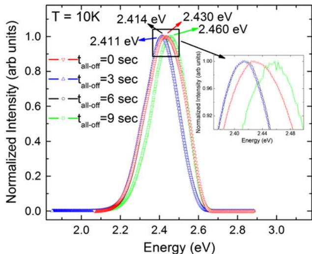
Fig. 5. Low-temperature PL of ZnTe/ZnSe QDs grown with different  $t_{\text{all-off}}$ .
