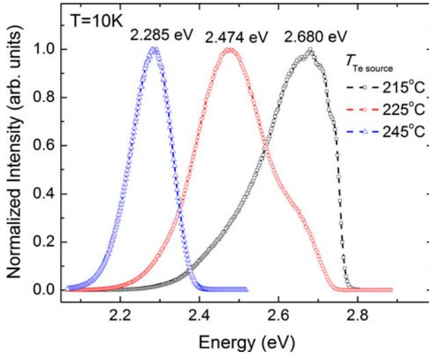
Fig. 2. Low-temperature PL of ZnTe/ZnSe QDs as a function of  $T_{\text{Te source}}$ .
