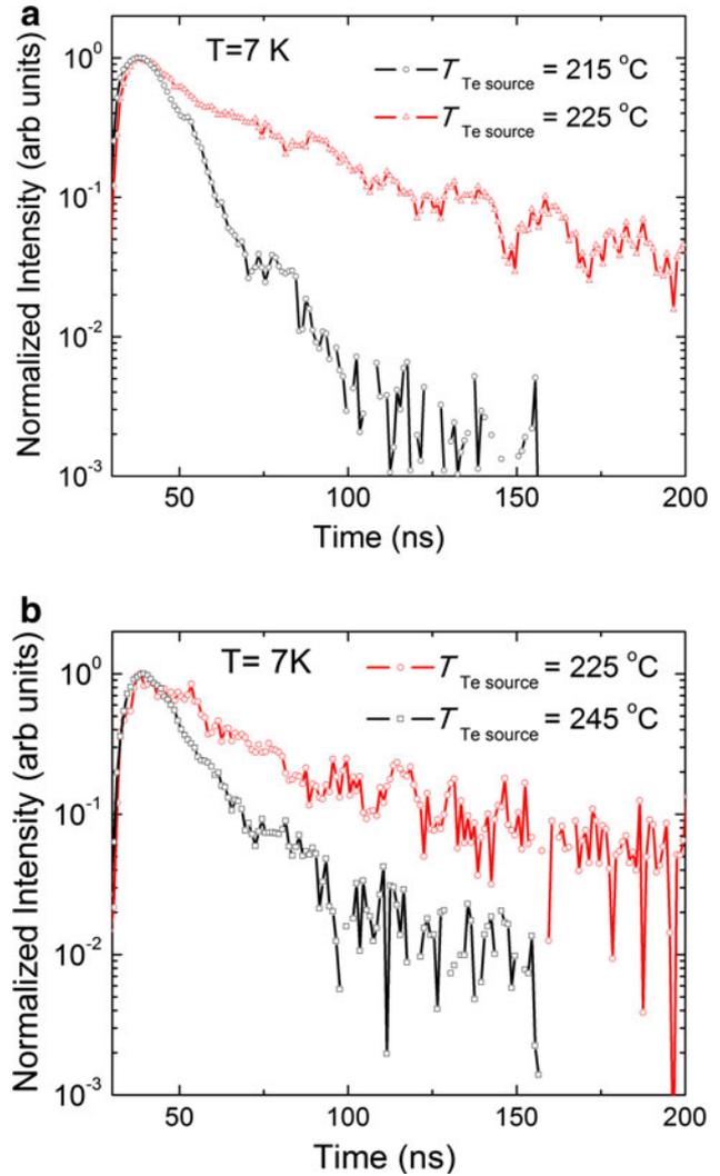
Fig. 4. (a) TRPL of ZnTe/ZnSe QDs grown with  $T_{\text{Te source}} = 215^\circ\text{C}$  and  $225^\circ\text{C}$ . (b) TRPL of ZnTe/ZnSe QDs for  $T_{\text{Te source}} = 225^\circ\text{C}$  and  $245^\circ\text{C}$ .
