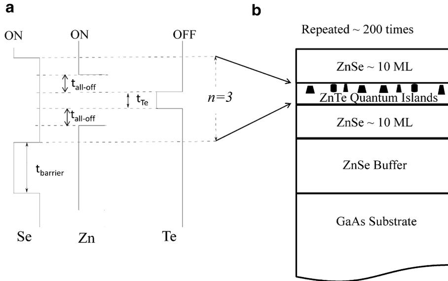
Fig. 1. Schematics of (a) shutter sequence for sample growth, and (b) sample structure.
