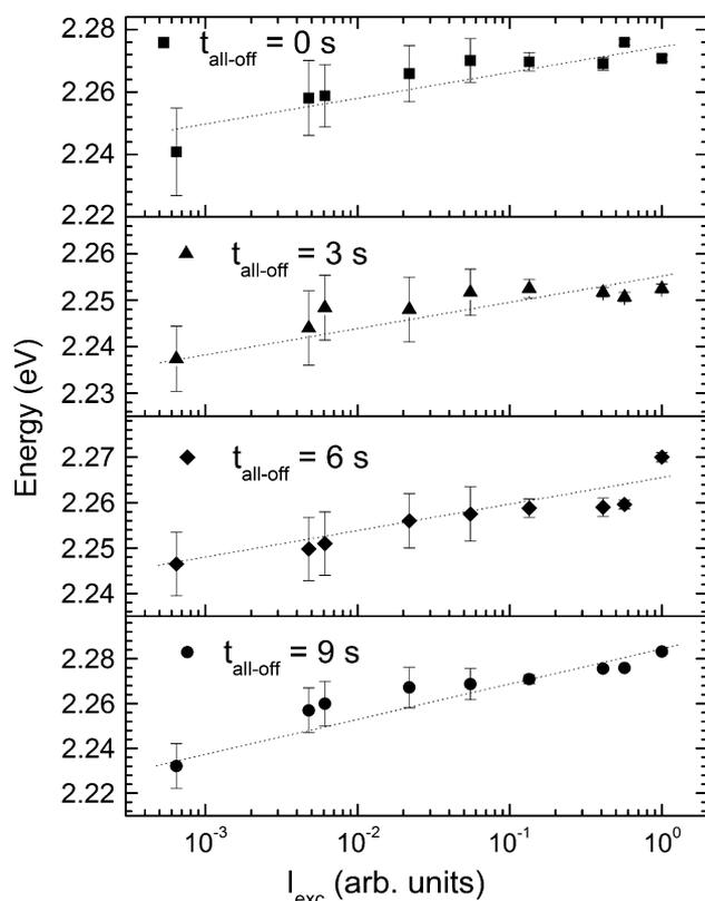
Fig. 6. Excitation intensity ( $I_{exc}$ ) dependence of the emission energy at 20% height of the peak on the low-energy side for samples in series II for different  $t_{all-off}$ . Dotted lines are guides to the eye.
