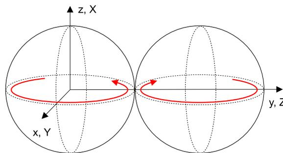
**Fig. 1** Configuration of a two-sphere system and possible coordinate systems. *Arrowed lines* show schematically two single-sphere fundamental modes
