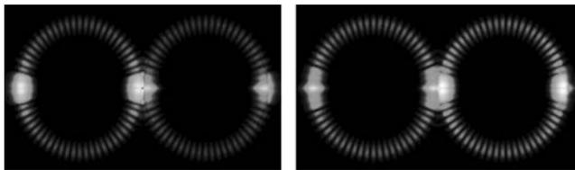
**Fig. 5** Distribution of the field in the regime of weak coupling for the lower frequency (left-hand figure) and the higher frequency (right-hand figure) resonances of the double-peak spectrum shown in Fig. 2c
