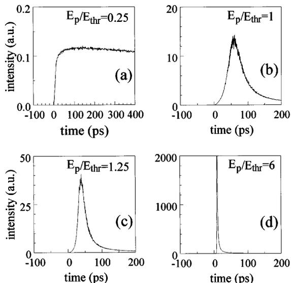
Fig. 2. Emission profiles from the Monte Carlo simulations for  $l = 18 \mu\text{m}$  and  $l_a = 140 \mu\text{m}$ . Emission for a pump energy (a) below threshold ( $0.12 \mu\text{J}$ ), (b) at threshold ( $0.47 \mu\text{J}$ ), (c) slightly above threshold ( $0.59 \mu\text{J}$ ), and (d) far above threshold ( $2.8 \mu\text{J}$ ).
