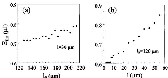
Fig. 3. Calculated threshold pump energy versus (a)  $l_a$  for fixed  $l = 30 \mu\text{m}$  and (b)  $l$  for fixed  $l_a = 120 \mu\text{m}$ .
