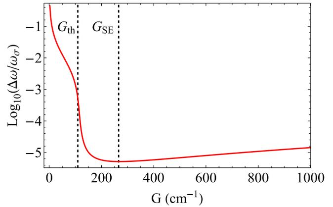
FIG. 6. The dependence of the linewidth of the lasing mode on gain.
