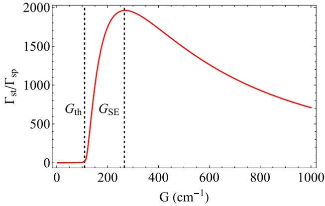
FIG. 5. The ratio of rates of stimulated and spontaneous transitions for the mode with the lowest generation threshold,  $\Gamma_{st}^0/\Gamma_{sp}^0$ , as a function of the gain coefficient of the active medium. The vertical dotted lines show the threshold gain coefficient,  $G_{th}$ , and the gain coefficient, at which the ratio  $\Gamma_{st}/\Gamma_{sp}$  has a maximum.
