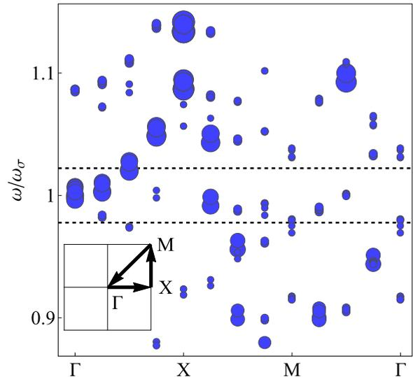
FIG. 2. Eigenmodes of a plasmonic DFB laser at the coordinates  $\Gamma X M \Gamma$ . The size of a dot reflects the value of the  $Q$  factor,  $\omega/(2\gamma_i)$ , of the respective mode. Horizontal dashed lines show the amplification linewidth of dye molecules. The inset shows the irreducible Brillouin zone with the  $\Gamma X M \Gamma$  path.
