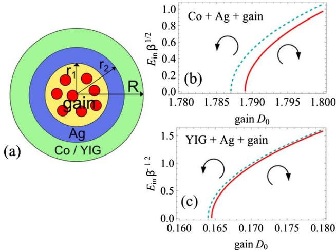
Fig. 2. (a) Alternative design of the MO spaser allowing for low-threshold spasing. (b), (c) Amplitudes of spasing modes versus gain for Co + Ag and YIG + Ag spasers, respectively.
