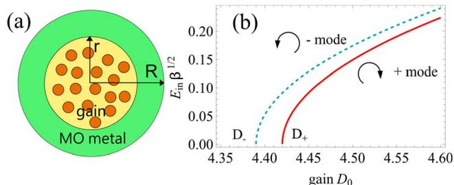
Fig. 1. (a) Schematic drawing of the suggested composite core-shell MO spaser. (b) Amplitudes of spasing modes of the MO spaser versus gain near the bifurcation point.
